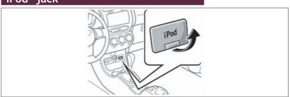
By inserting the standard iPod® connector cable into the iPod® jack, you can charge the iPod® battery, control the iPod® functions using the car audio unit and listen to music from your iPod® through the vehicle's speaker system.
